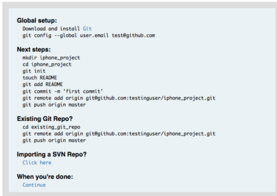
Figure 4.7: Instructions for a new repository
